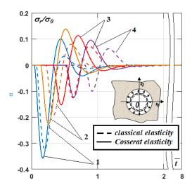
Figure 3 Relative radial stresses in the polymer foam with tunnel cavity
