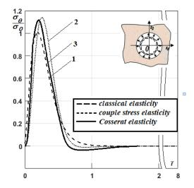
Figure 2 Relative hoop stresses on the boundary of the cavity in polymer foam
